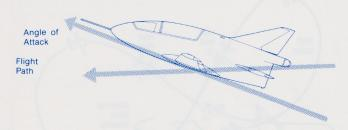
At slow speeds a pilot uses a large angle of attack to maintain level flight. At high speeds a pilot uses a small angle of attack. When flying your AcroJet, if the plane appears to be flying level but the VVI indicates you a altitude, you need to adjust your angle of attack. Briefly push the stick forward or back (i.e., pitch down or up) to change your angle of attack.
